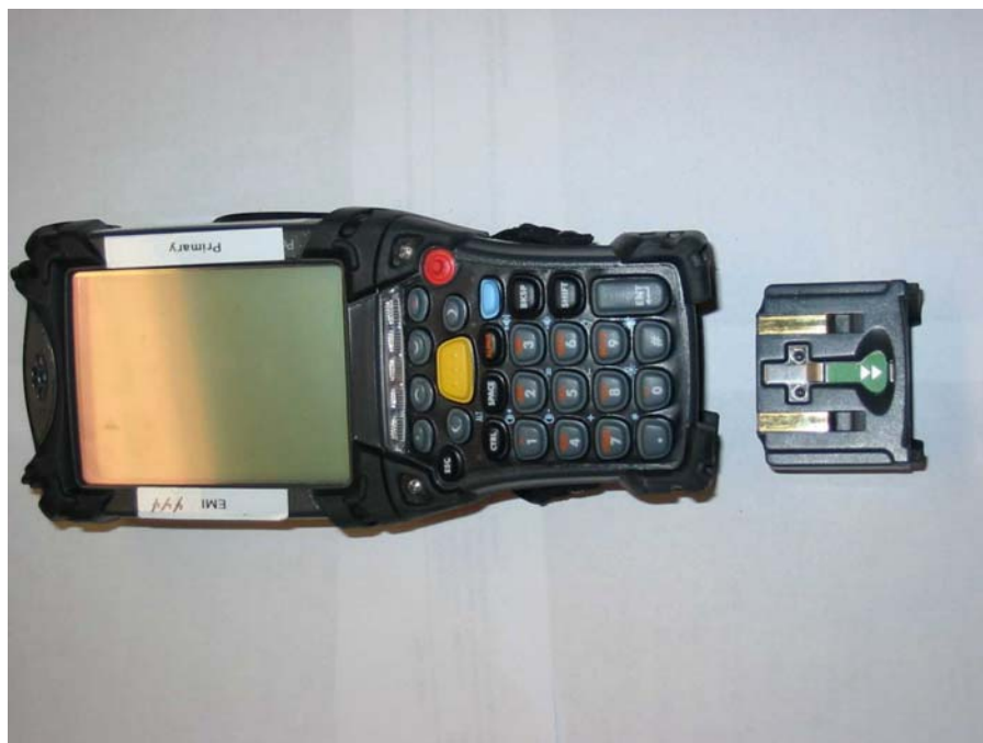
Figure 4 – MC9063 with Battery Removed
