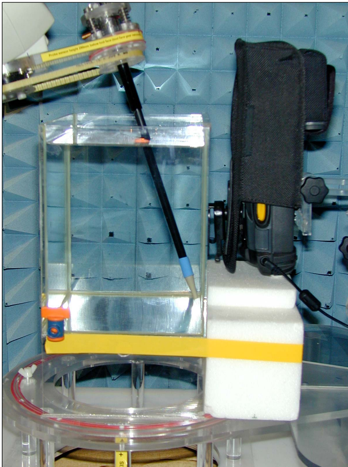
Figure 6 – With the device in a Mobile Computer Holster with the LCD facing out from the rear of the Holster and the belt Clip in contact with the flat phantom
