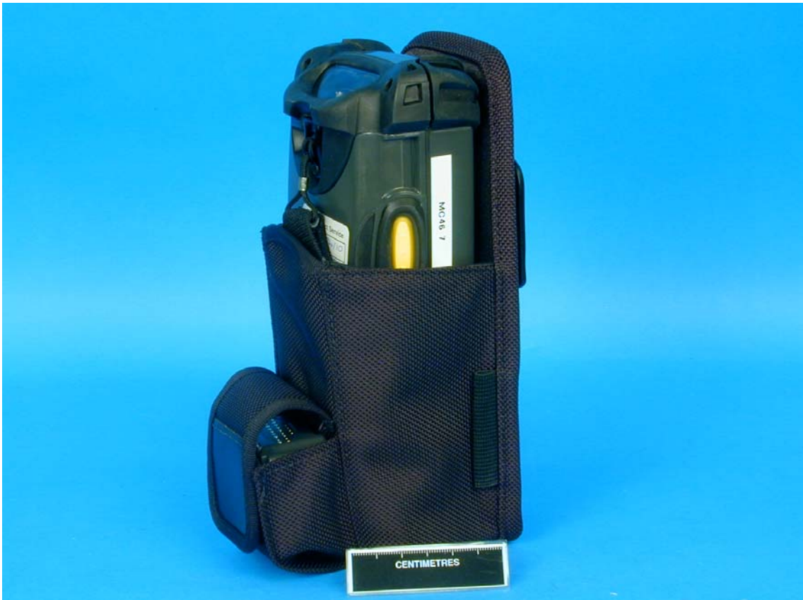
Figure 51. Device placed in correct position with the MC9062 Mobile Computer Holster with LCD facing rear of Holster.
