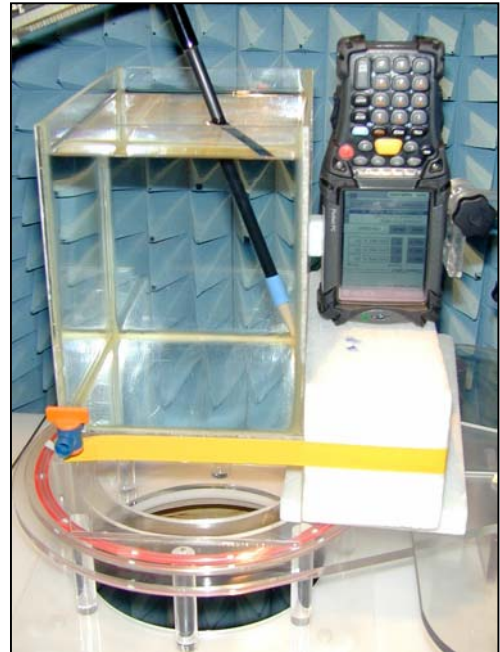
Figure 46. Positional photograph of the MC9062 Right-hand side at 1.0cm from Phantom side
