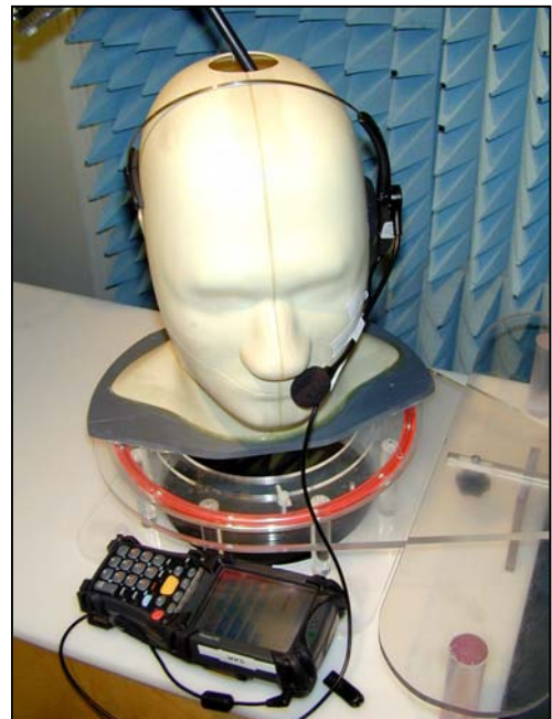
Figure 48. Positional photograph of the MC9062 with Headset connected and placed against the SAM Phantom in the left-hand Cheek Position
