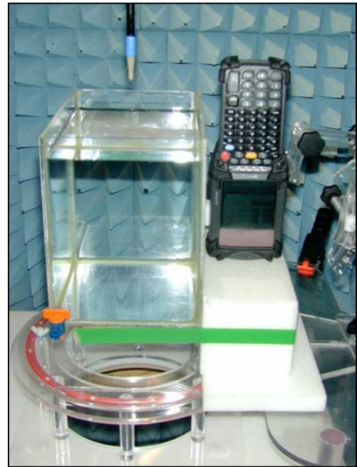
Figure 38. Positional photograph of the MC9062 Right-hand side at 1.0cm from Phantom side
