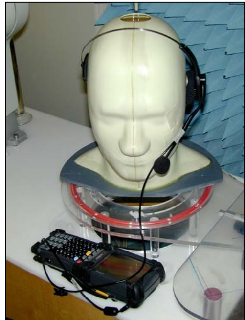
Figure 42. Positional photograph of the MC9062 with Headset connected and placed against the SAM Phantom in the left-hand Cheek Position
