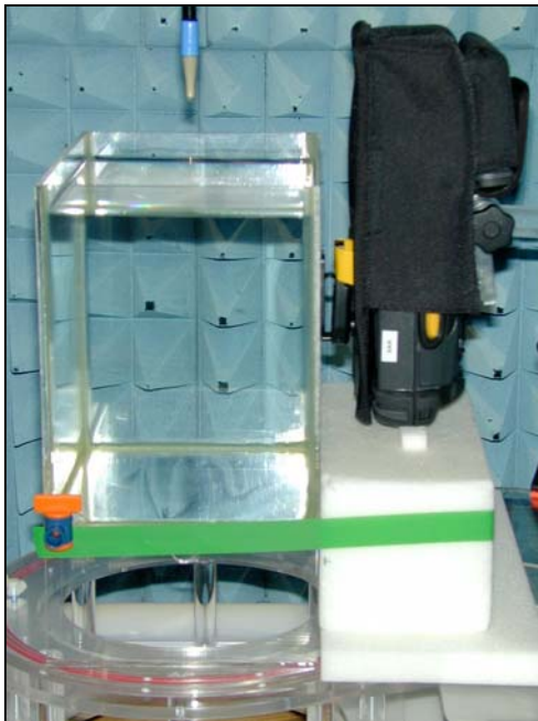
Figure 41. Positional photograph of the MC9062 with the device in a Mobile Computer Holster with the LCD side facing the rear of the Holster and the belt Clip in contact with the flat phantom.
