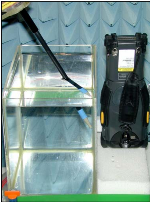
Figure 39. Positional photograph of the MC9062 left-hand side at 1.0cm from Phantom side
