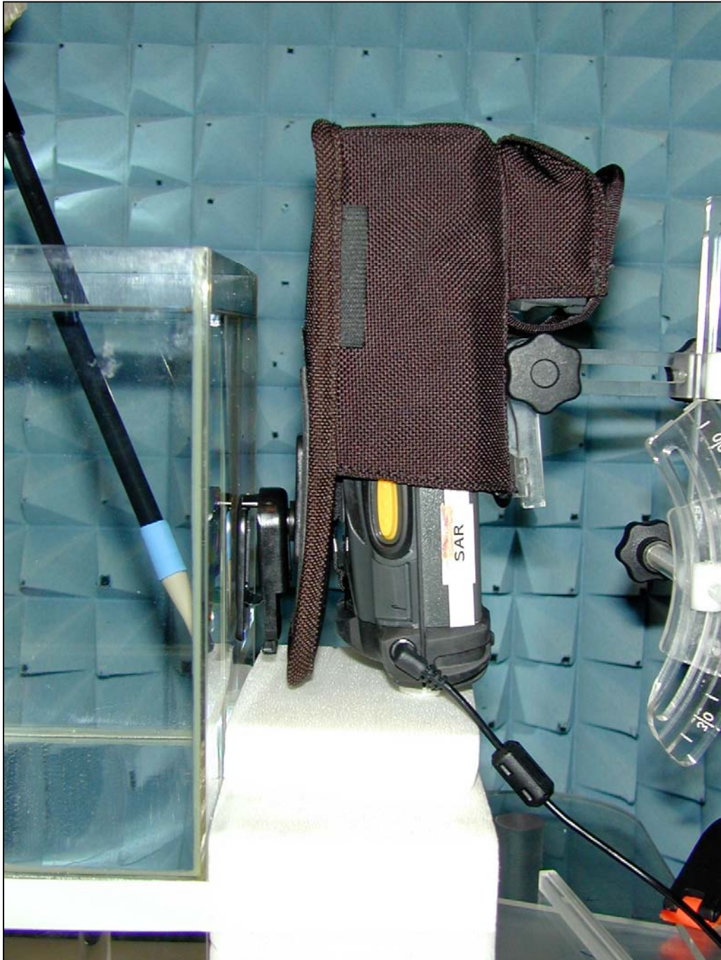
Figure 8 – With the device in a Mobile Computer Holster with the LCD side facing out from the rear of the Holster and the belt Clip in contact with the flat phantom
