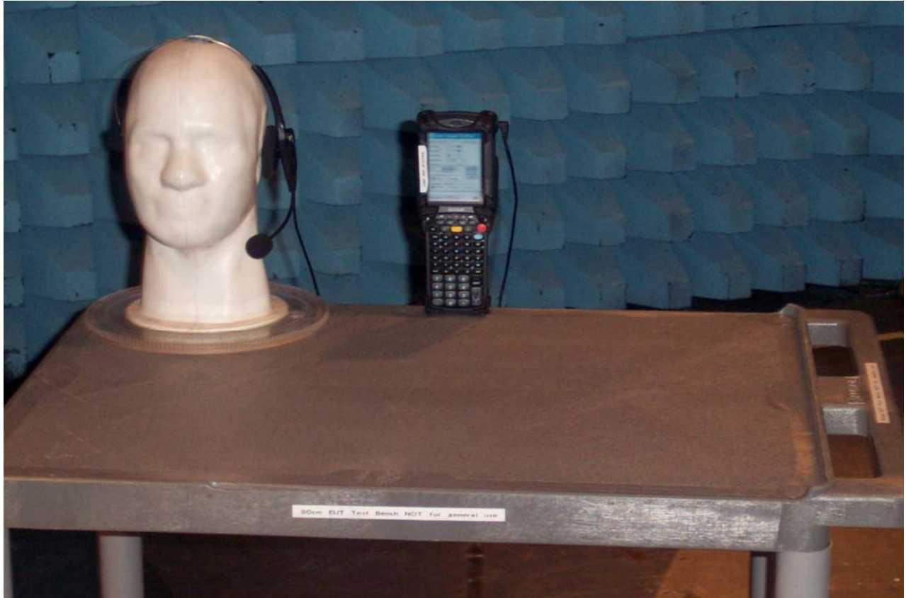
Spurious Radiated Emissions Set Up Photograph
