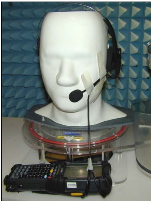
Figure 27. Positional photograph of the MC9060 with Headset connected and placed against the SAM Phantom in the left-hand Cheek Position.
