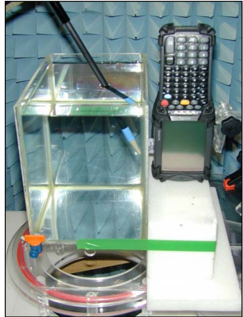
Figure 26. Positional photograph of the MC9060 Right-hand side at 1.0cm from Phantom side
