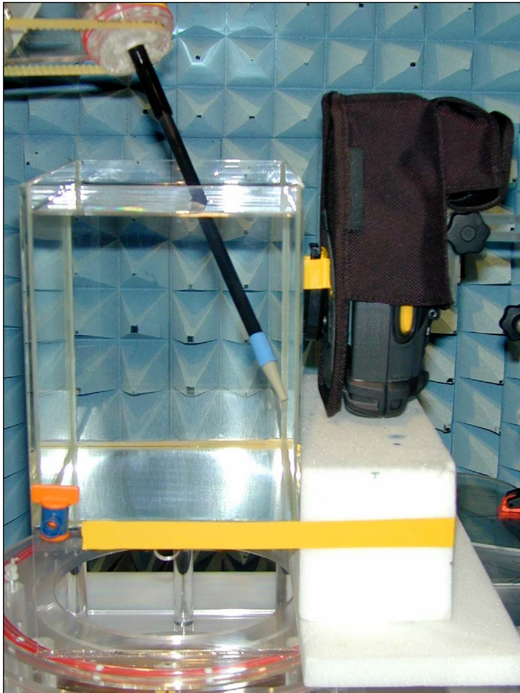
Figure 6 – With the device in a Mobile Computer Holster With the LCD side facing the rear of the Holster and the belt Clip in contact with the flat phantom
