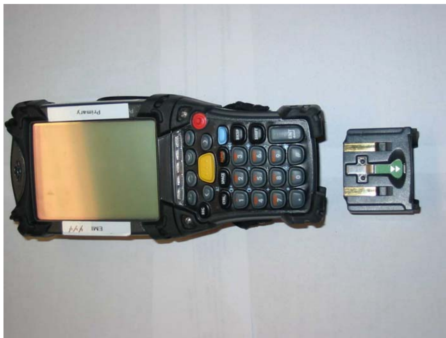
Figure 4 – MC9063 with Battery Removed
