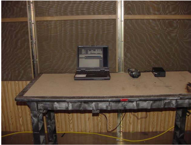
AC Line conducted emission setup photographs
