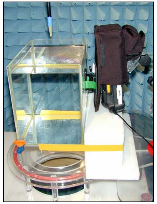
Figure 40. Positional photograph of the MC9062 With the device in a Mobile Computer Holster With the Rear side facing the rear of the Holster and the belt Clip in contact with the flat phantom.
