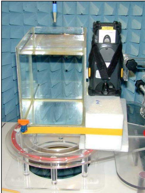
Figure 37. Positional photograph of the MC9062 left-hand side at 1.0cm from Phantom side
