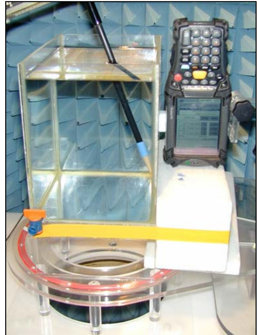
Figure 51. Positional photograph of the MC9062 Right-hand side at 1.0cm from Phantom side
