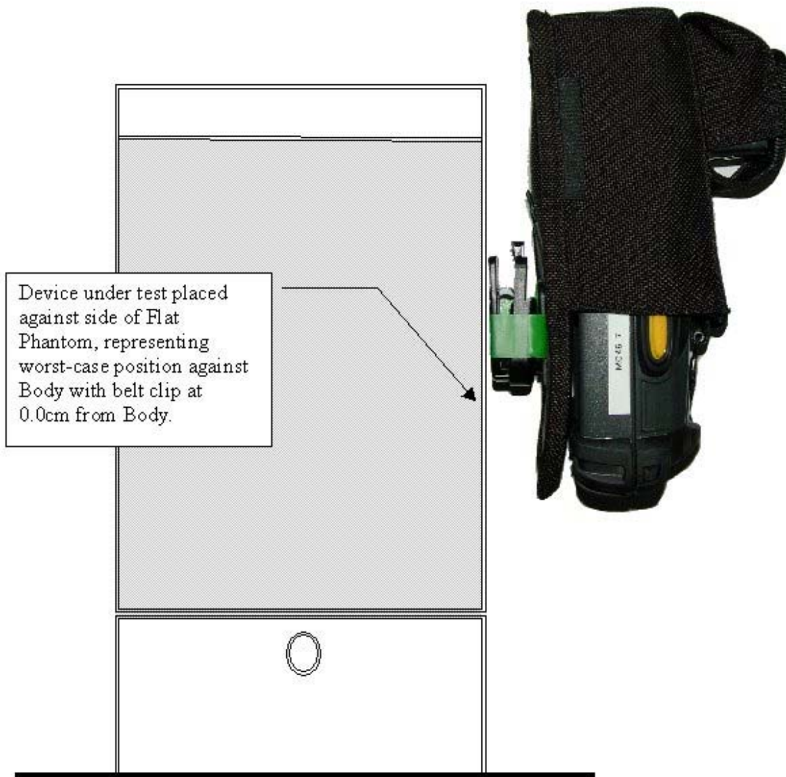
Figure 14. – MC9062 Test position for body assessment in declared normal use position; holster belt clip 0.0 cm from phantom side.
