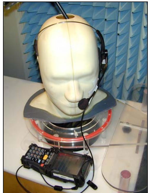
Figure 53. Positional photograph of the MC9062 with Headset connected and placed against the SAM Phantom in the left-hand Cheek Position
