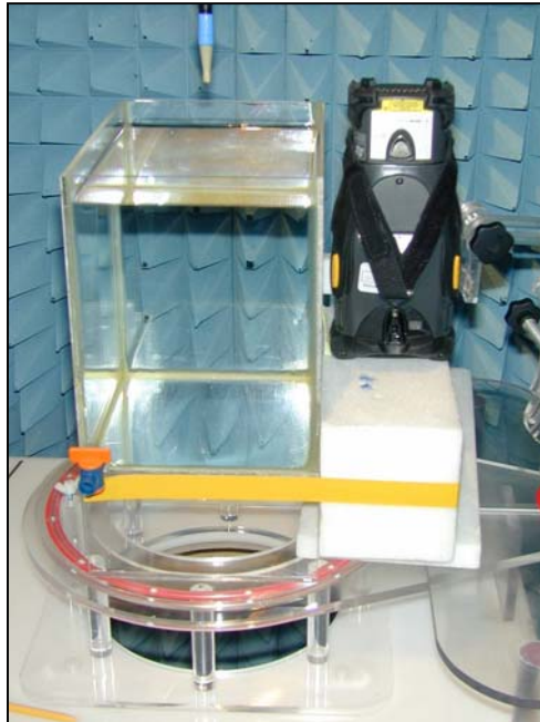
Figure 50. Positional photograph of the MC9062 left-hand side at 1.0cm from Phantom side
