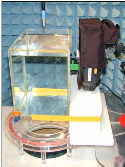
Figure 52. Positional photograph of the MC9062 With the device in a Mobile Computer Holster With the LCD side facing the rear of the Holster and the belt Clip in contact with the flat phantom.
