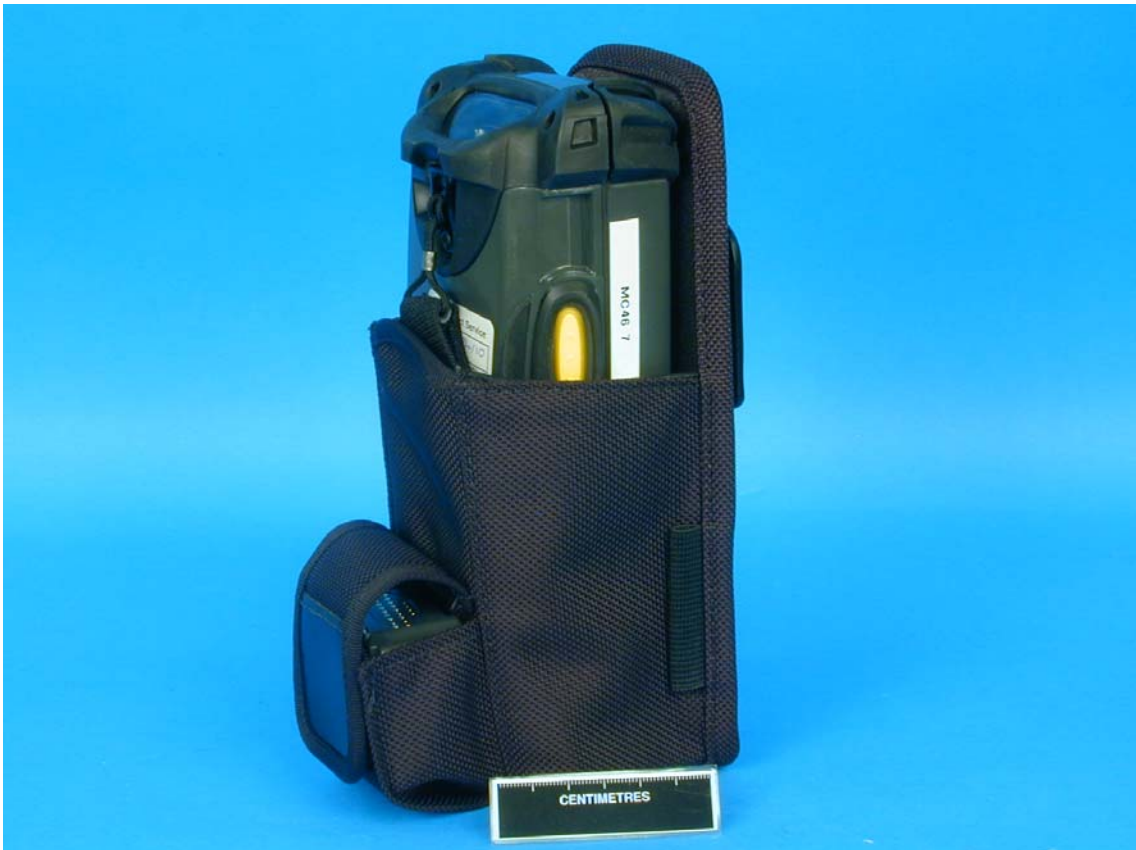
Figure 56. Device placed in correct position with the MC9062 Mobile Computer Holster with LCD facing rear of Holster.
