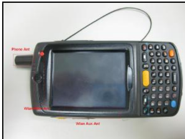
DESCRIPTION OF ANTENNA LOCATION
