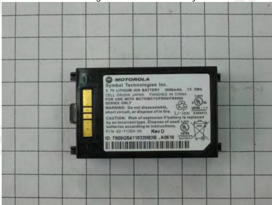
Fig.6 Back view of Battery
