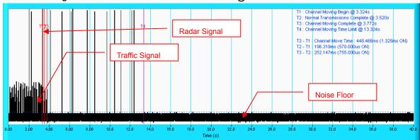
**NOTE:** T1 denotes the start of Channel Move Time upon the end of the last Radar burst. T2 denotes the data transmission time of 200ms from T1. T3 denotes the 10 second from T1 to observe the aggregate duration of transmissions.
