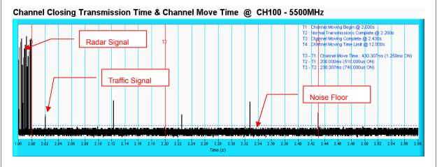
**NOTE:** An expanded plot for the device vacates the channel in the required 200ms.
