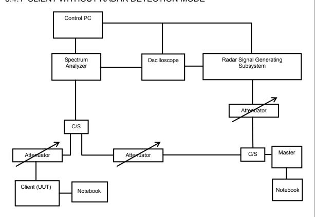
The UUT is a U-NII Device operating in Client mode without radar detection. The radar test signals are injected into the Master Device.
