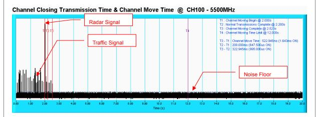
**NOTE:** T1 denotes the start of Channel Move Time upon the end of the last Radar burst. T2 denotes the data transmission time of 200ms from T1. T3 denotes the 10 second from T1 to observe the aggregate duration of transmissions.
