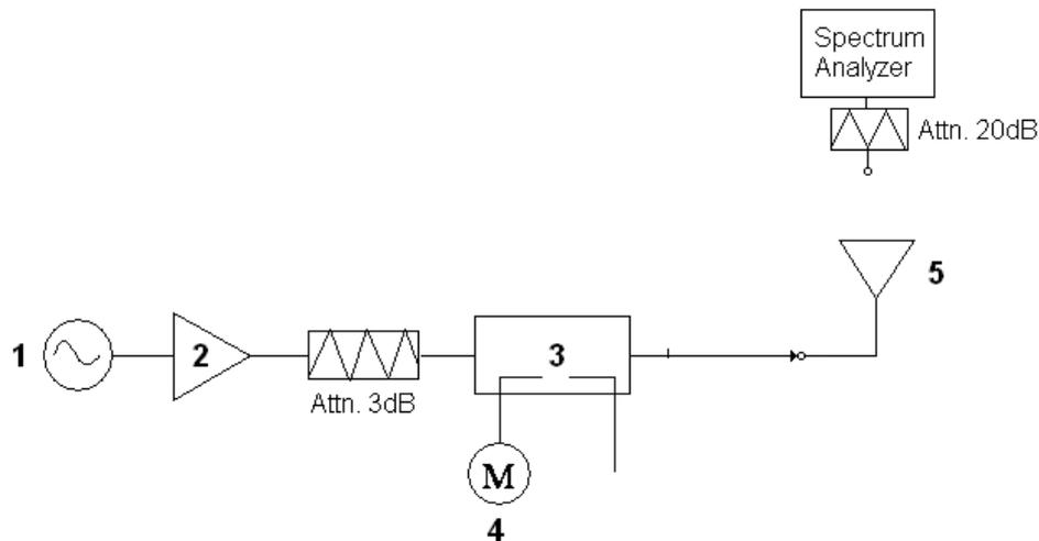
**Fig. 8.1 System Calibration**
