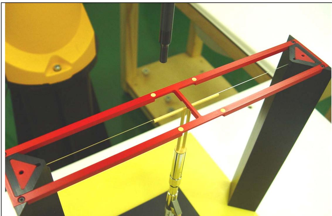
**Fig 7.2 Dipole Setup**
