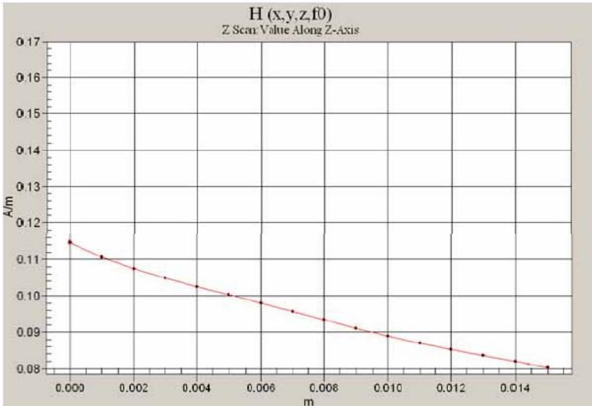
**Fig. 5.5 Z-Axis Scan at maximum point above a typical wireless device for H-field**
