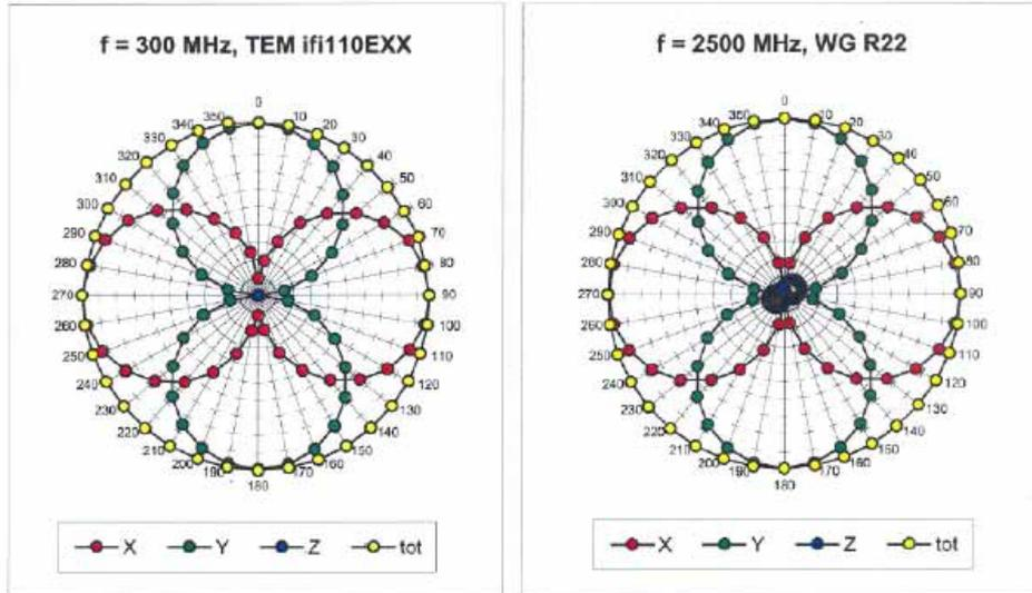
Receiving Pattern ( $\phi$ ),  $\vartheta = 0^\circ$
