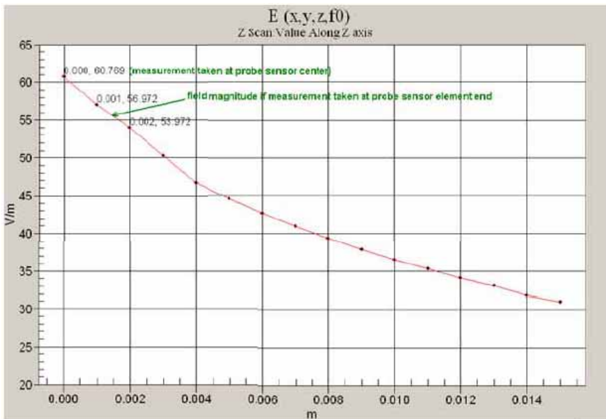
Fig. 5.4 Z-Axis Scan at maximum point above a typical wireless device for E-field
