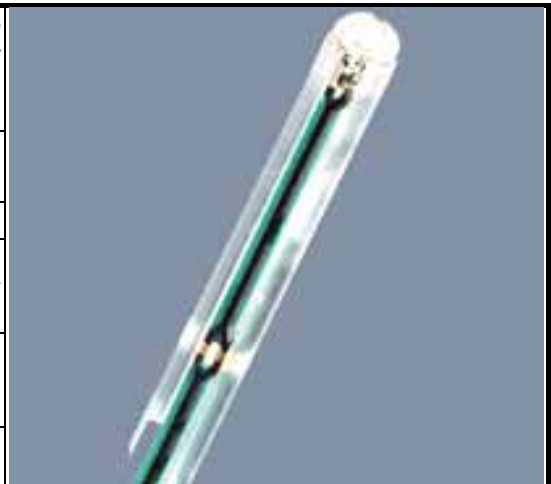
Fig. 5.3 H-field Free-space Probe
