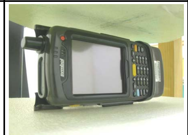
F: EUT with gun in body position The left of the EUT face to the phantom with 15mm-separation distance.
