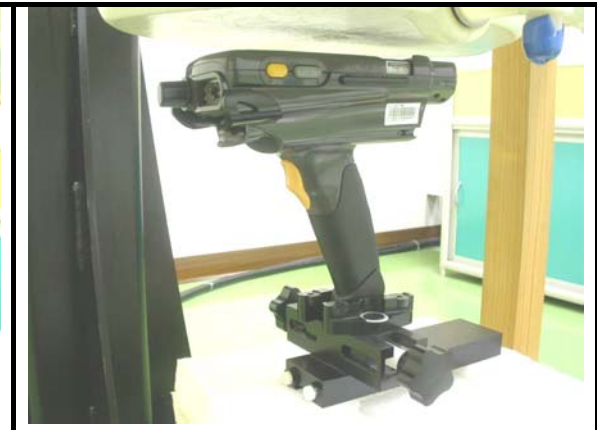
D: EUT with gun in body position The front of the EUT face to the phantom with 15mm-separation distance.
