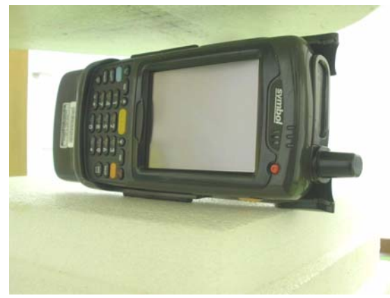
H: EUT with gun in body position The right of the EUT face to the phantom with 15mm-separation distance.
