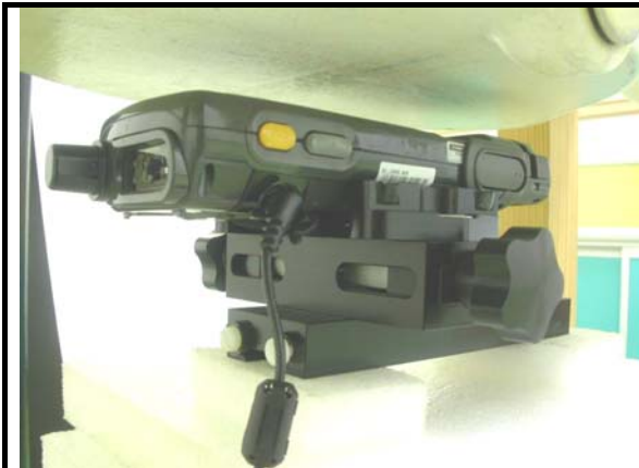
C: EUT with reader in body position The front of the EUT face to the phantom with 15mm-separation distance.
