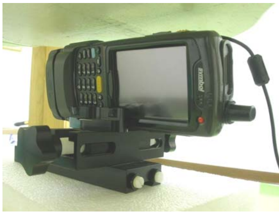
G: EUT with reader in body position The right of the EUT face to the phantom with 15mm-separation distance.
