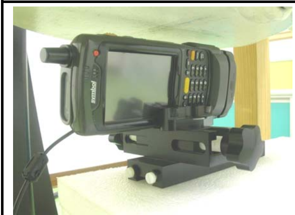
E: EUT with reader in body position The left of the EUT face to the phantom with 15mm-separation distance.
