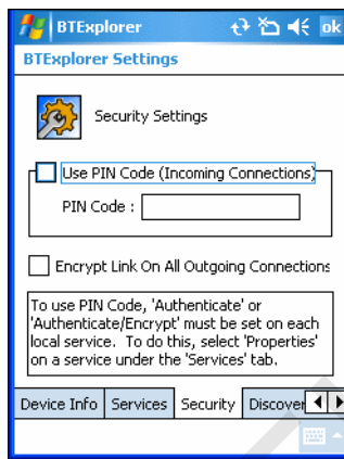
Figure 3-43 BTExplorer Settings - Security Tab
