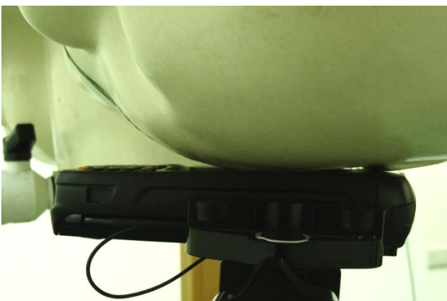
Left Cheek - DUT with Battery 1 + Scanner 2 + Keypad 2
