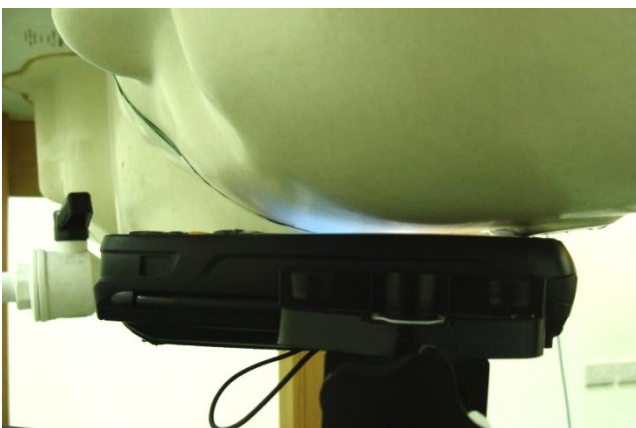
Left Cheek - DUT with Battery 2 + Scanner 2 + Keypad 3
