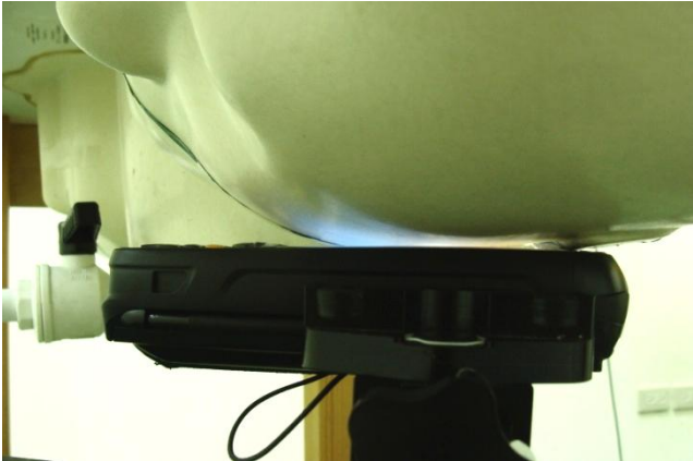
Left Cheek - DUT with Battery 2 + Scanner 1 + Keypad 3
