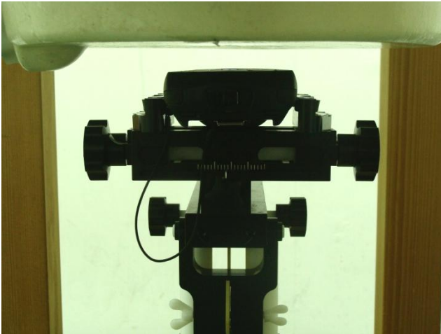
Face of the DUT with Battery 1 + Scanner 2 + Keypad 2 (with Phantom 1.5 cm Gap)
