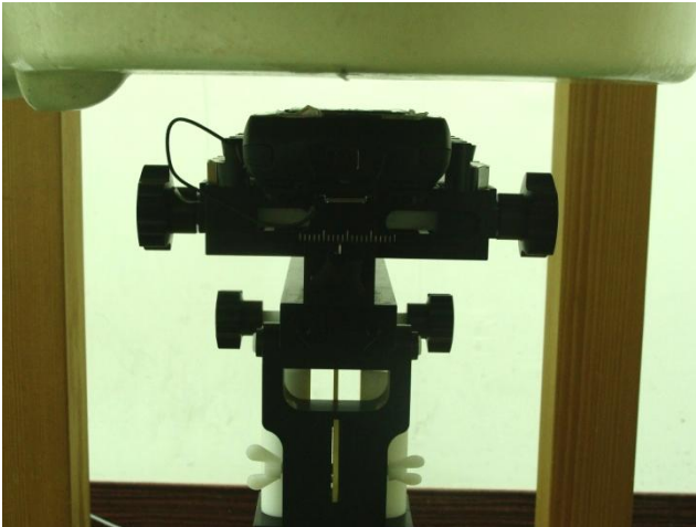
Face of the DUT with Battery 1 + Scanner 1 + Keypad 1 (with Phantom 1.5 cm Gap)
