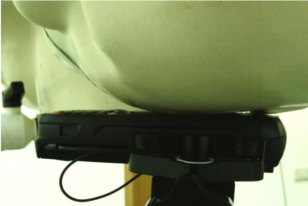
Left Cheek - DUT with Battery 1 + Scanner 1 + Keypad 2
