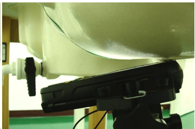
Left Tilted - DUT with Battery 1 + Scanner 1 + Keypad 3
