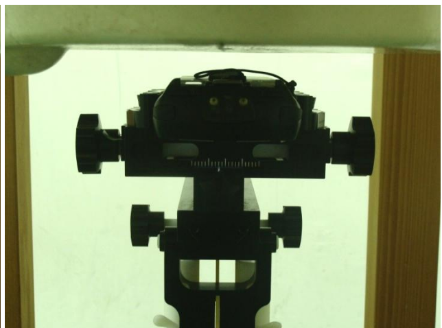
Bottom of the DUT with Battery 1 + Scanner 2 + Keypad 3 (with Phantom 1.5 cm Gap)
