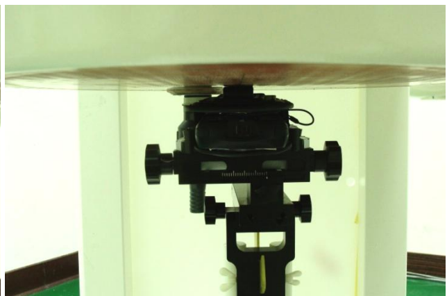
Bottom of the DUT with Battery 1 + Scanner 1 + Keypad 1 (Holster 2 with Phantom 0 cm Gap)
