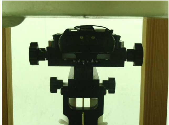
Bottom of the DUT with Battery 1 + Scanner 2 + Keypad 2 (with Phantom 1.5 cm Gap)
