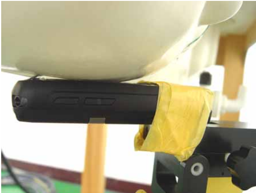
EUT with 2D Scanner + Battery 2 Right Cheek
