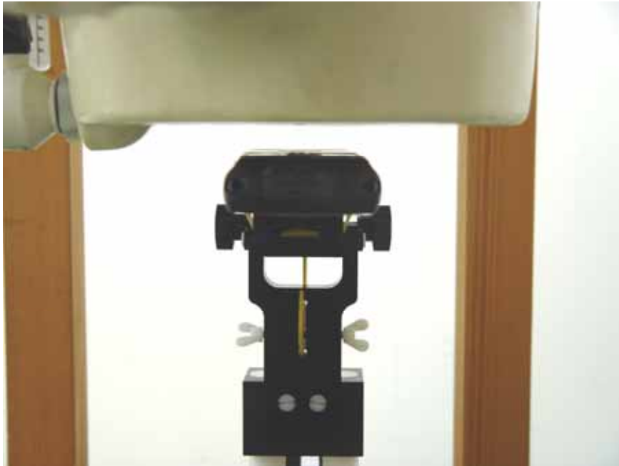
EUT with 2D Scanner + Battery 2 Bottom with 1.5cm Gap
