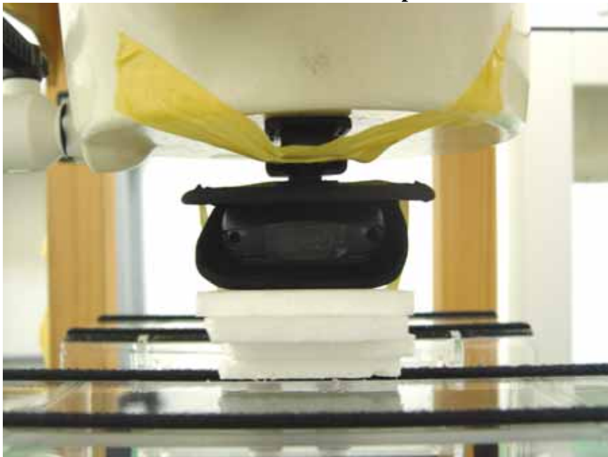
EUT with 2D Scanner and Holster 2 Face with 0cm Gap
