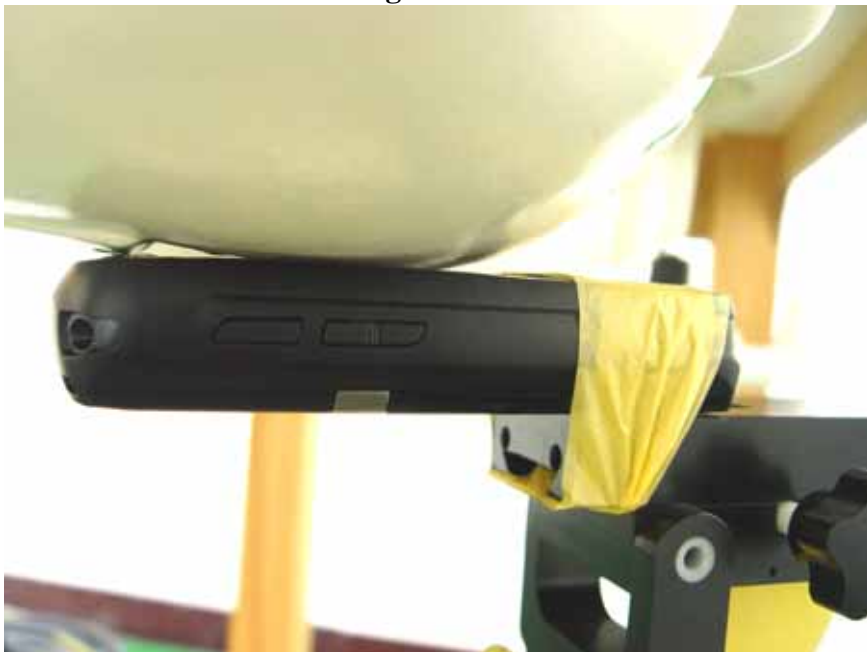
EUT with 1D Scanner + Battery 2 Right Cheek
