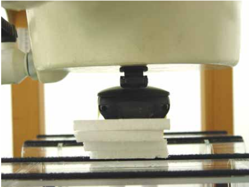
EUT with 2D Scanner and Holster 1 Face with 0cm Gap
