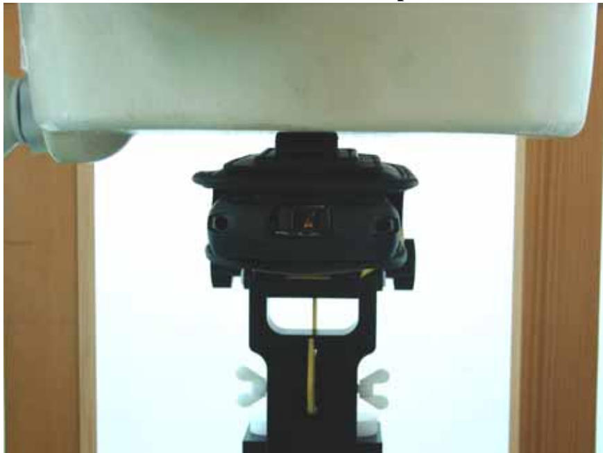
EUT with 2D Scanner and Holster 3 Bottom with 0cm Gap
