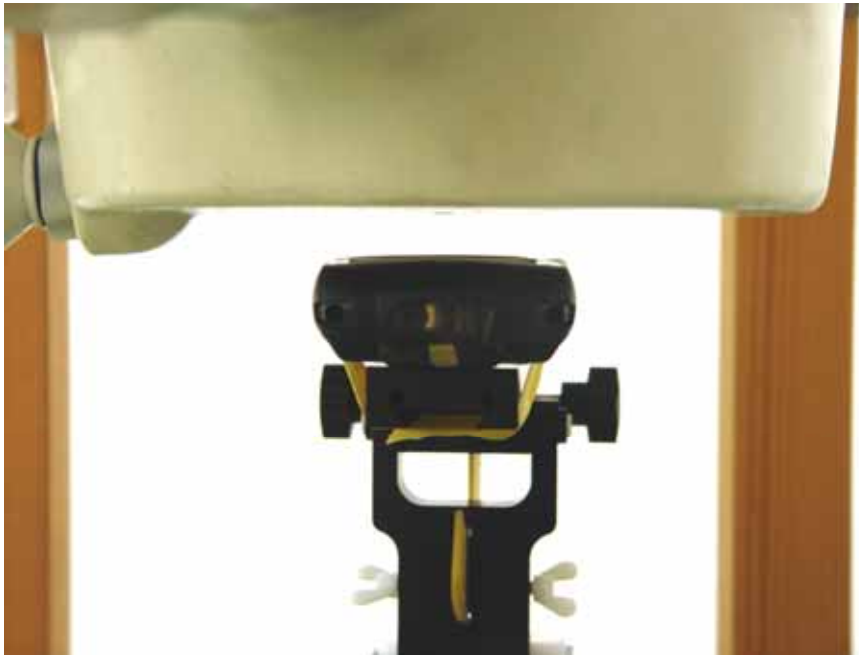
EUT with 1D Scanner + Battery 1 Face with 1.5cm Gap
