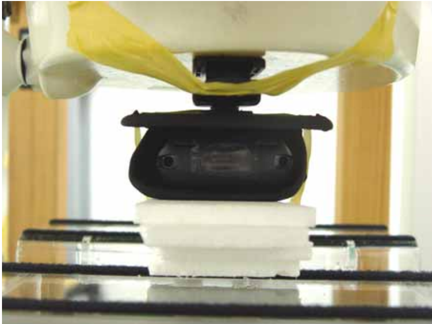
EUT with 2D Scanner and Holster 2 Bottom with 0cm Gap
