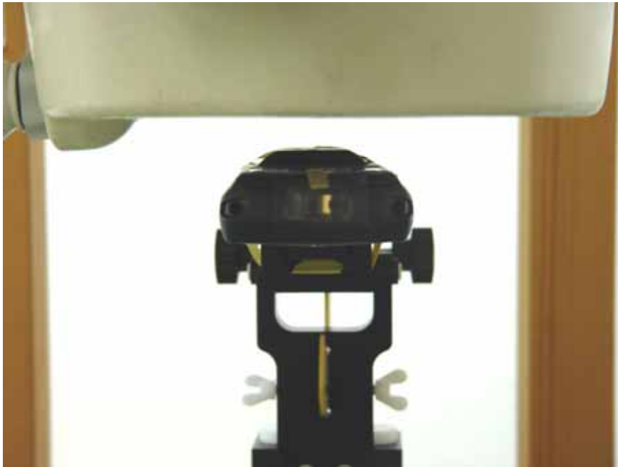
EUT with 1D Scanner + Battery 1 Bottom with 1.5cm Gap
