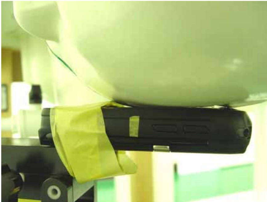
EUT with 1D Scanner + Battery 2 Left Cheek
