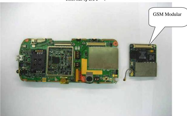
Internal of EUT – 5 (GSM Modular)
