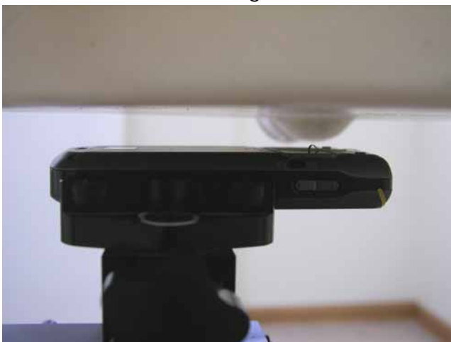
Fig.7 Body position- EUT back to flat phantom (testing in GPRS Mode)
