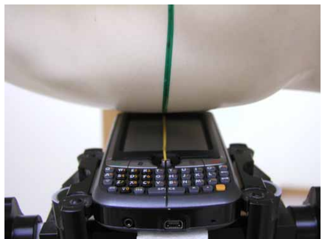
Fig.4 Right Head Section / Ear-Tilt Position(15°)
