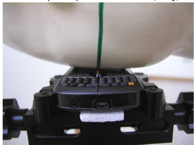
Fig.3 Right Head Section / Cheek-Touch Position
