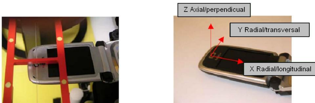
Figure 2. Photo of the device positioned under Test Arch and coordinate system
