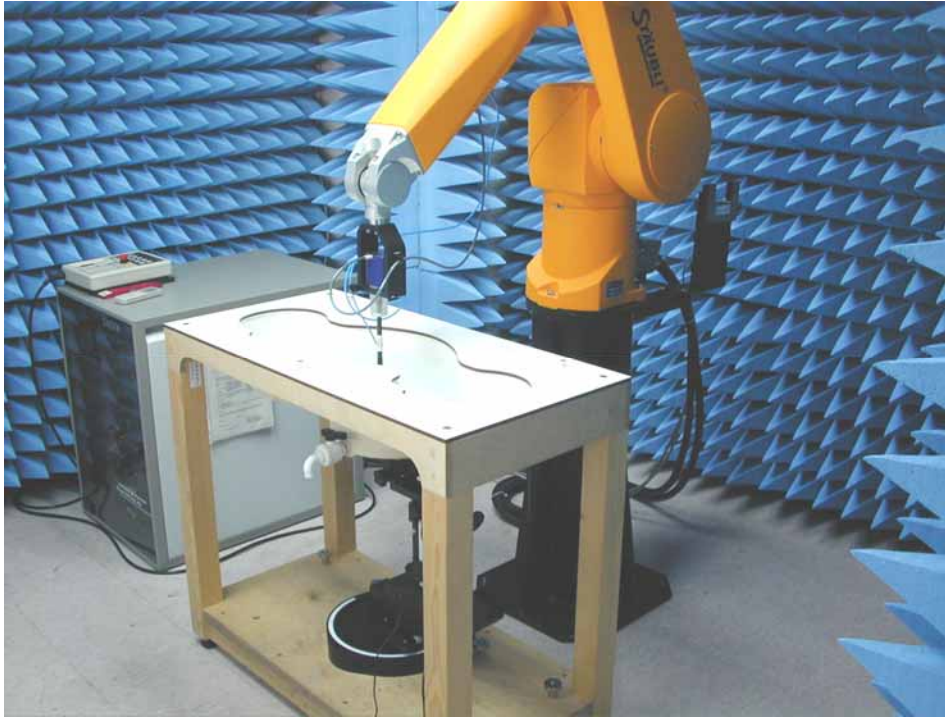
Fig.1 Photograph of the SAR measurement System
