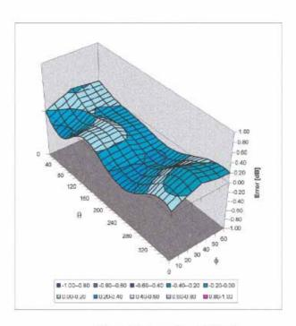
Spherical Isotropy Error < ± 0.4 dB
