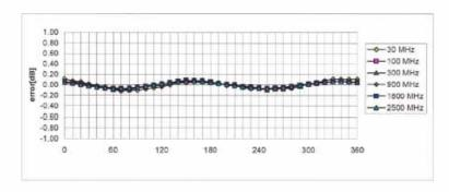
Axial Isotropy Error < ± 0.2 dB
