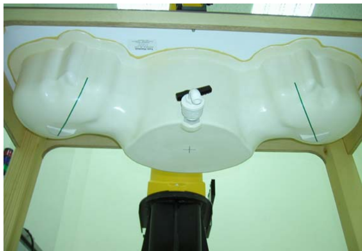
Fig. 5.4 Bottom view of twin phantom
