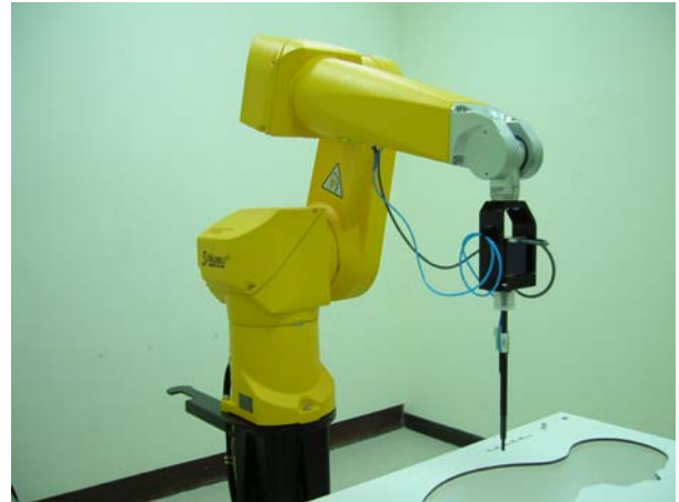
Fig. 5.2 Probe setup on robot
