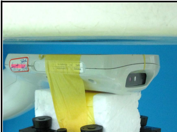
Body-worn Mode, Front Face of EUT with 1.0 cm Gap
