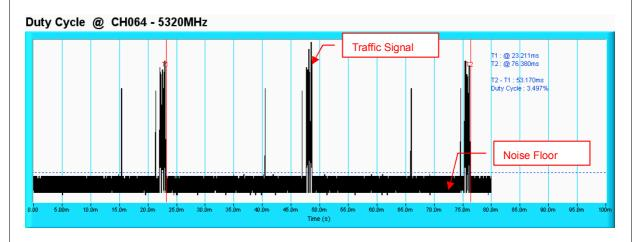
**NOTE:** T1 denotes the start of duty cycle period is  $0.023211^{th}$  second. T2 denotes the end of duty cycle period is  $0.07638^{th}$  second. T2 – T1= 0.5317 seconds. Duty Cycle = 3.497%
