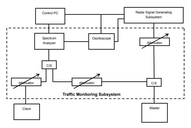
The test transmission will always be from the Master Device to the Client Device. While the Client device is set up to associate with the Master device and play the WAV file from Master device, the designated WAV test file and instructions are located at: <a href="http://ntiacsd.ntia.doc.gov/dfs/">http://ntiacsd.ntia.doc.gov/dfs/</a>.
