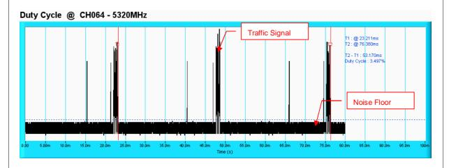
**NOTE:** T1 denotes the start of duty cycle period is  $0.023211^{th}$  second. T2 denotes the end of duty cycle period is  $0.07638^{th}$  second. T2 – T1= 0.5317 seconds. Duty Cycle = 3.497%
