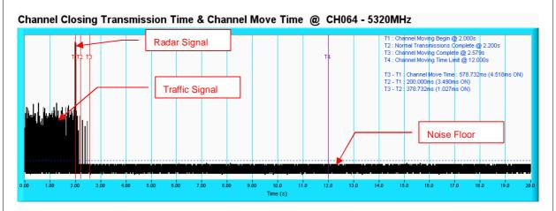
**NOTE:** T1 denotes the start of Channel Move Time upon the end of the last Radar burst. T2 denotes the data transmission time of 200ms from T1. T3 denotes the 10 second from T1 to observe the aggregate duration of transmissions.
