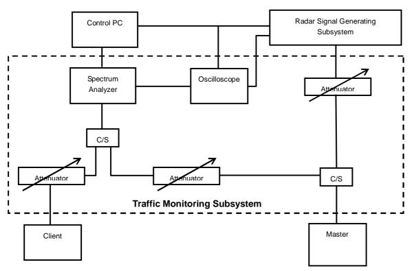
The test transmission will always be from the Master Device to the Client Device. While the Client device is set up to associate with the Master device and play the WAV file from Master device, the designated WAV test file and instructions are located at: <a href="http://ntiacsd.ntia.doc.gov/dfs/">http://ntiacsd.ntia.doc.gov/dfs/</a>. The test with WAV file, because MPEG2 file cannot be played with the EUT.
