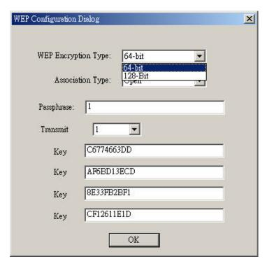
**WEP Encryption Type -** The 64-bit and 128-bit WEP encryption algorithm is provided by RSA and uses RC4 encryption/decryption, which is based on a 40-bit key, 104-bit key and 128-bit key respectively. Select the same encryption used by the Access Point in order to interoperate.
