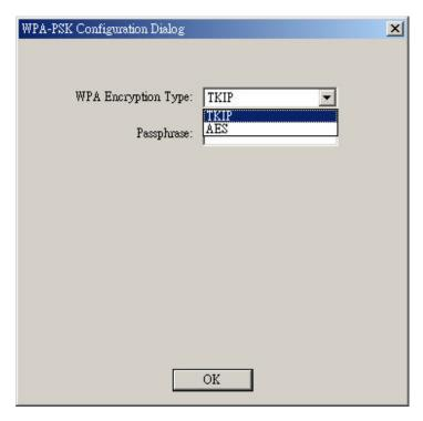
**WPA Encryption Type -** TKIP and AES are the actual encryption algorithms used on the packets
