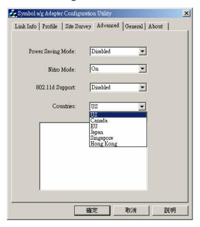
Use the Advanced page to configure the **Power Saving Mode.** There are 3 options: **Disabled, Dynamic,** and **Maximum.** If selecting Disabled, the device does not conserve power. Select Maximum, to conserve as much power as possible. If Dynamic is selected, the device constantly switches between the power-saving state and awake state.
