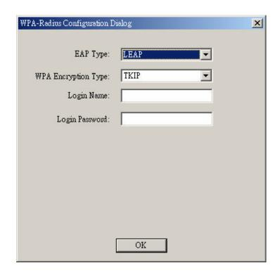
**WPA Encryption Type-** TKIP and AES are the encryption algorithms used on the packets
