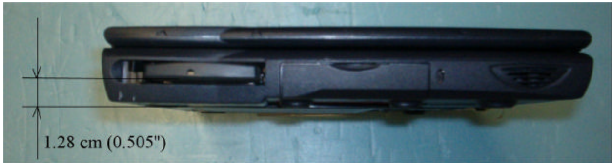
c. Side view showing the Cardbus Adapter edge.
