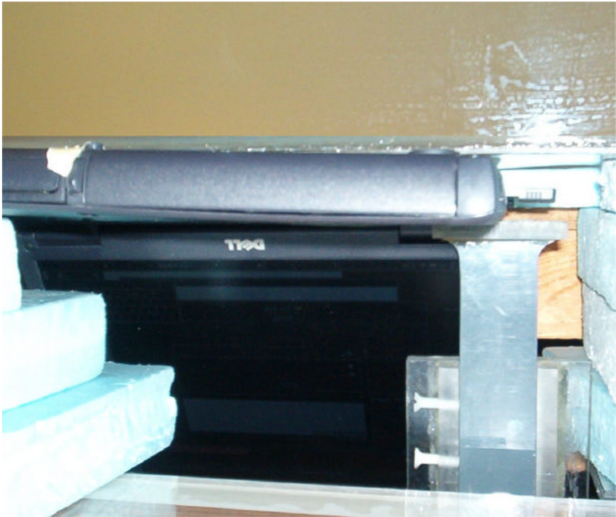
Fig. 2. Photograph of the bottom of the Dell Model PP01L Host Computer with Symbol Wireless Networker 802.11a/g CardBus Adapter Model LA-5030 pressed against the bottom of the planar phantom. This Configuration 1 – Laptop position for SAR testing.
