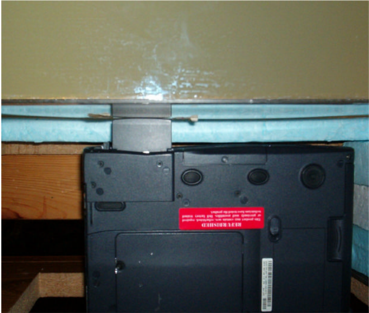
Fig. 3. Photograph of the Dell Model PP01L Host Computer at 90° with the edge of the Symbol Wireless Networker 802.11a/g CardBus Adapter Model LA-5030 pressed against the bottom of the planar phantom. This is Configuration 2 for SAR testing and represents the case of a bystander at a distance of 0 cm from the edge of the Cardbus Adapter.
