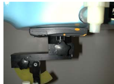
Figure 18. Hand SAR Test Setup
