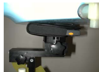
Figure 17. Body SAR Test Setup
