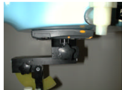
Figure 18. Hand SAR Test Setup
