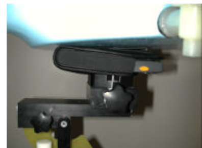
Figure 17. Body SAR Test Setup
