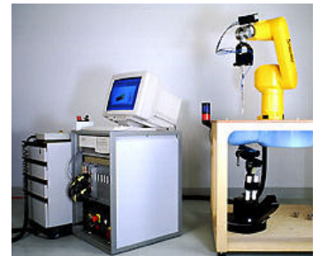
Fig. 1 SAR Test Setup
