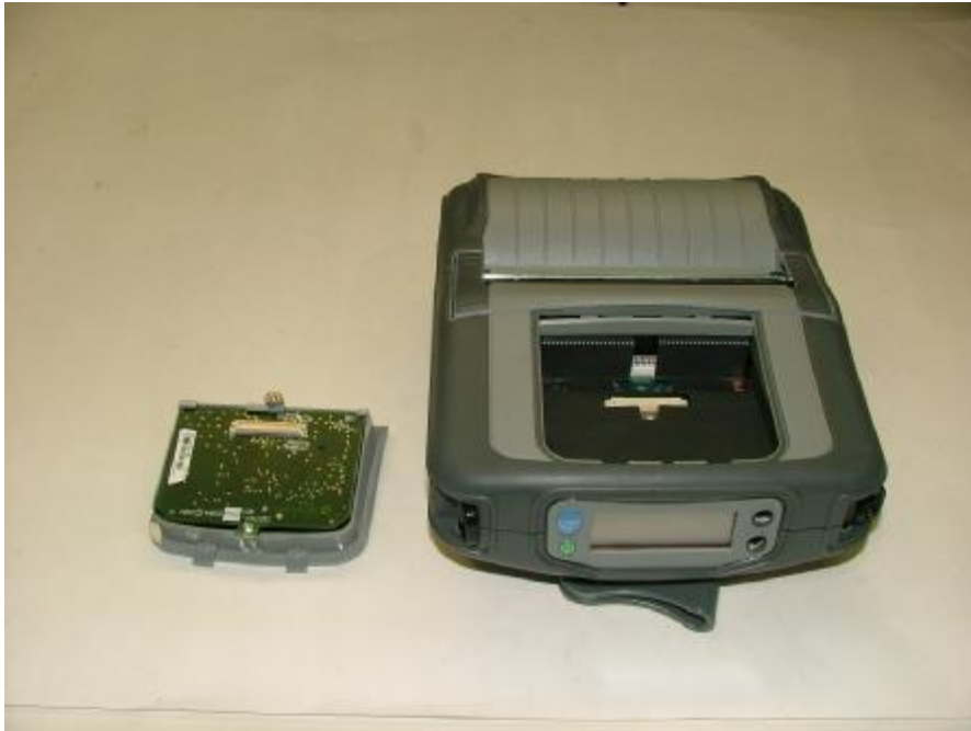
RF Carrier Board Removed
