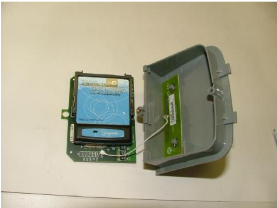
RF Carrier Board with H9PLA4137 Installed
