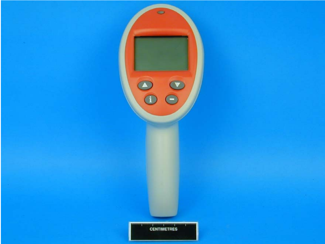
Figure 20. Front view of the Symbol PS3050 Terminal.
