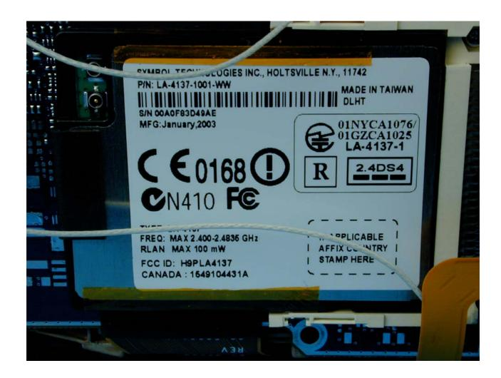
Photograph 12 MC9050 View of Symbol LA-4137 RLAN Compact Flash Card
