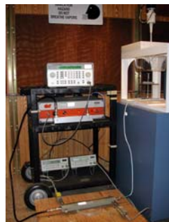
Figure 12.1 Dipole Validation Test Setup
