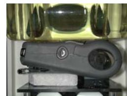
Figure 14.2 Hand SAR Test Setup
