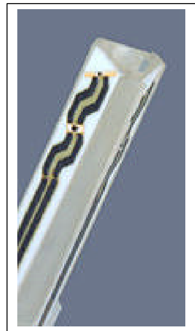
Inside view of ET3DV6 E-field Probe
