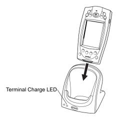
The Terminal Charge LED turns red (may take up to one minute) to indicate charging, then green when the battery is fully charged. The terminal's battery is fully charged after approximately 2 1/2 hours.
