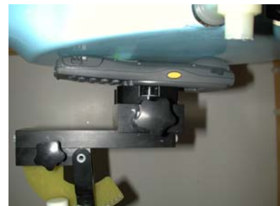
Figure 18. Hand SAR Test Setup
