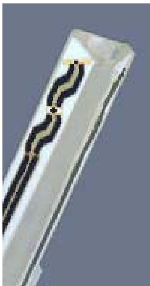
Fig. 5. ET3DV6 E-field Probe
