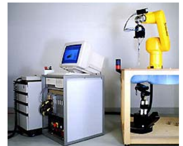
Fig. 1 SAR Test Setup
