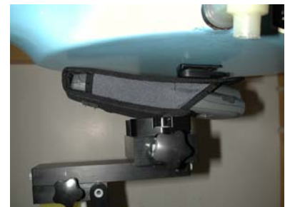
Figure 17. Body SAR Test Setup w/Holster
