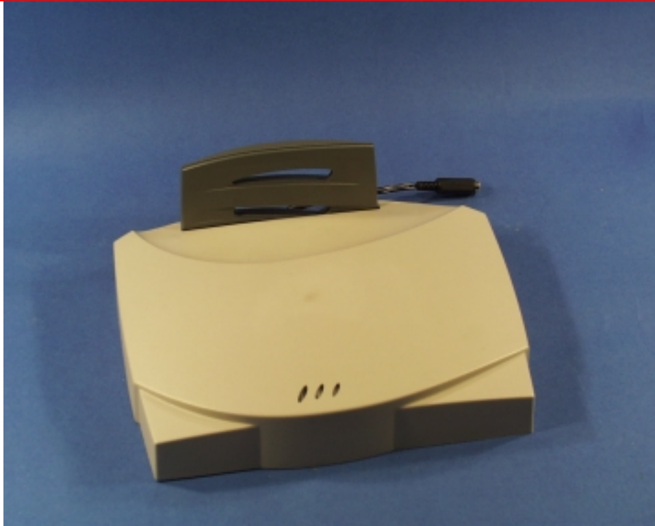
Access point table top configuration
