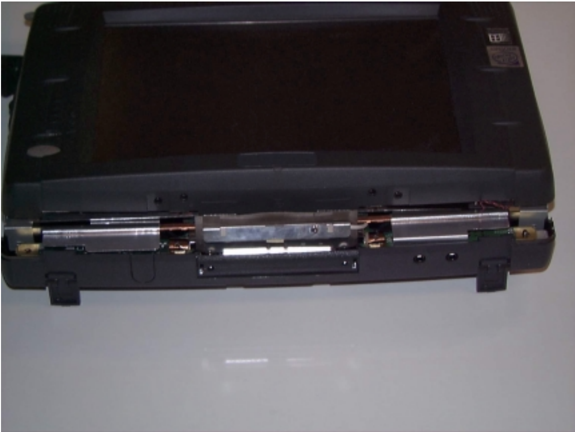
Antenna Installed in Device
