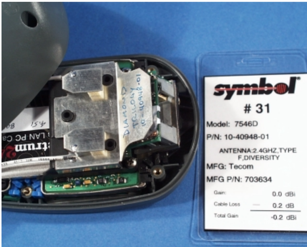
Antenna Installed in Device
