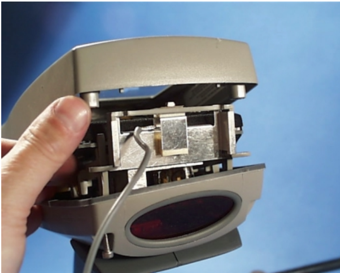
Antenna Installed in Device
