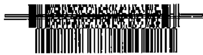
Aim the single scan line at the center of the 2D portion
