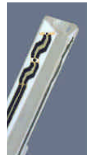
Figure 3.2 Probe Thick-Film Technique
