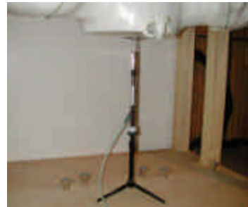
Figure 12.1 Dipole Validation Test Setup
