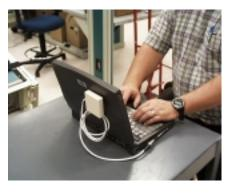
The Plane antenna is 0 dBi omni-directional in azimuth plane. It would typically be mounted on a ceiling but could mount on top of a computer. In
