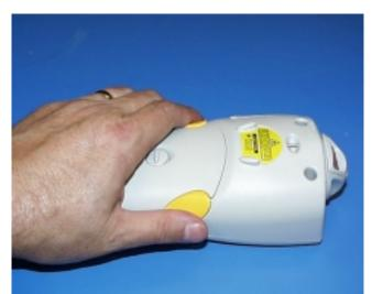
to hand and wrist tissues. Scanning button locations keep the users hand away from the antenna element to enhance device range and RF safety. Since the 6140 hand held computer has the same gain as the as the WWC 1049 but is not used as close as the
