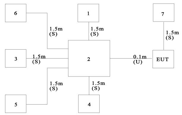
m: Length in metersS: Shielded cableU: Unshielded cable
